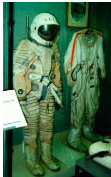
Figure B.1-8. The Berkut EVA suit used by A. Leonov.
