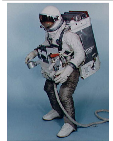
Figure B.3-2 AMU as configured for Gemini 9. (NASA photo S66-33167).
