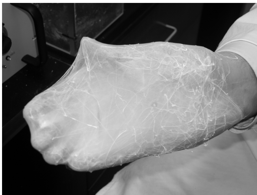
Figure 2. EVOH electrospun directly onto a human hand.
