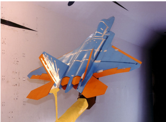
13.5% Scale F-22 in LaRC Transonic Dynamics Tunnel
