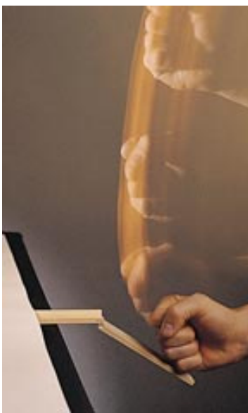
Figure 4. The newsprint is used to snap a board in this demonstration of the force exerted by atmospheric pressure.
