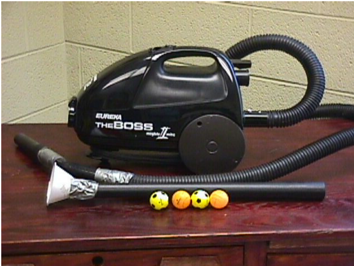
Figure 2. The Bernoulli vacuum. The vacuum blows out rather than sucks in and the special attachment has a funnel duct-taped to one end. The ping-pong balls remain trapped in the funnel due to the Bernoulli effect.
