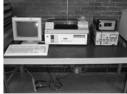
Figure 16. B-H test setup [8] and Walker Scientific AH 400 hysteresis plotting equipment
