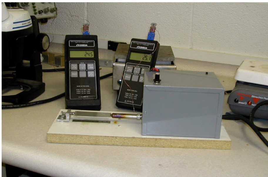
Figure 1. Equipment used in this experiment. The home-made thermal conductivity apparatus is shown in the front and the two thermistors in the back.
