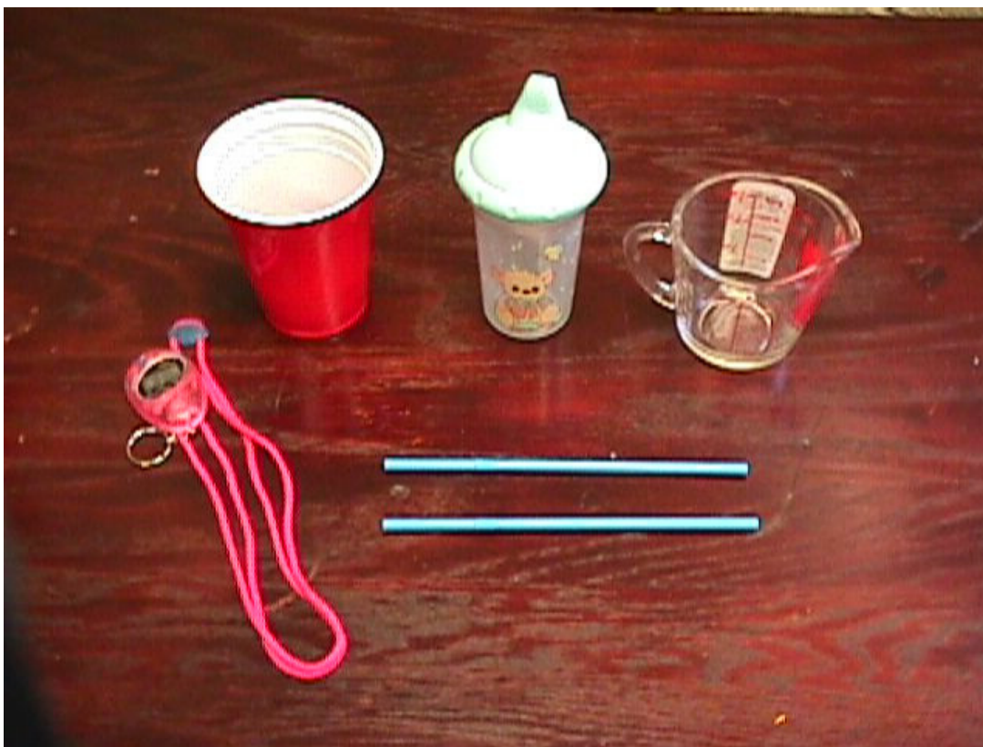
Figure 3. The measuring cup and stop watch are used to estimate the volume flow rate and hence the Reynolds number in this race to see who can achieve the highest Reynolds number in a straw.
