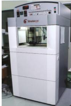
The Stratasys 3-D Modeler with retrofitted high-pressure extrusion head
