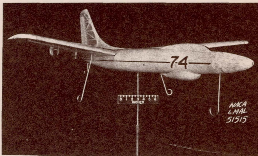
Figure 3.- Photographs of \frac{1}{20} -scale model of the Consolidated Vultee XB-53 airplane.
