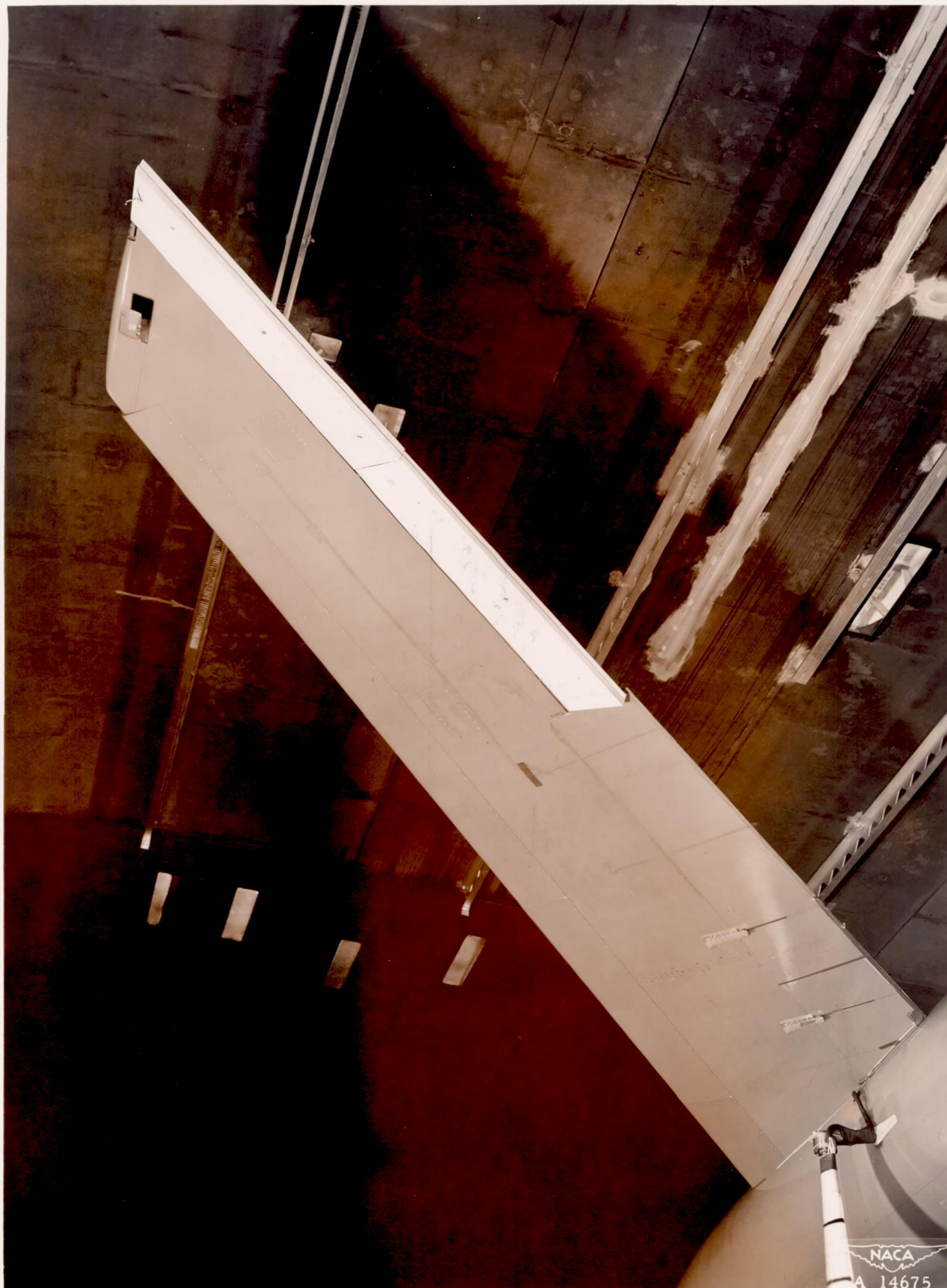
(i) Close-up of the lower surface of the left wing showing the slab-sided elevons.
