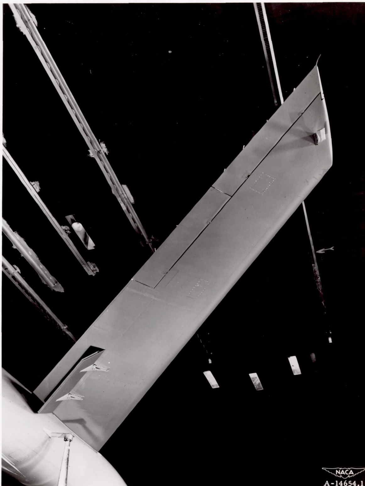
(c) Close-up of the lower surface of the right wing showing the trailing-edge split flaps deflected 45^\circ .
