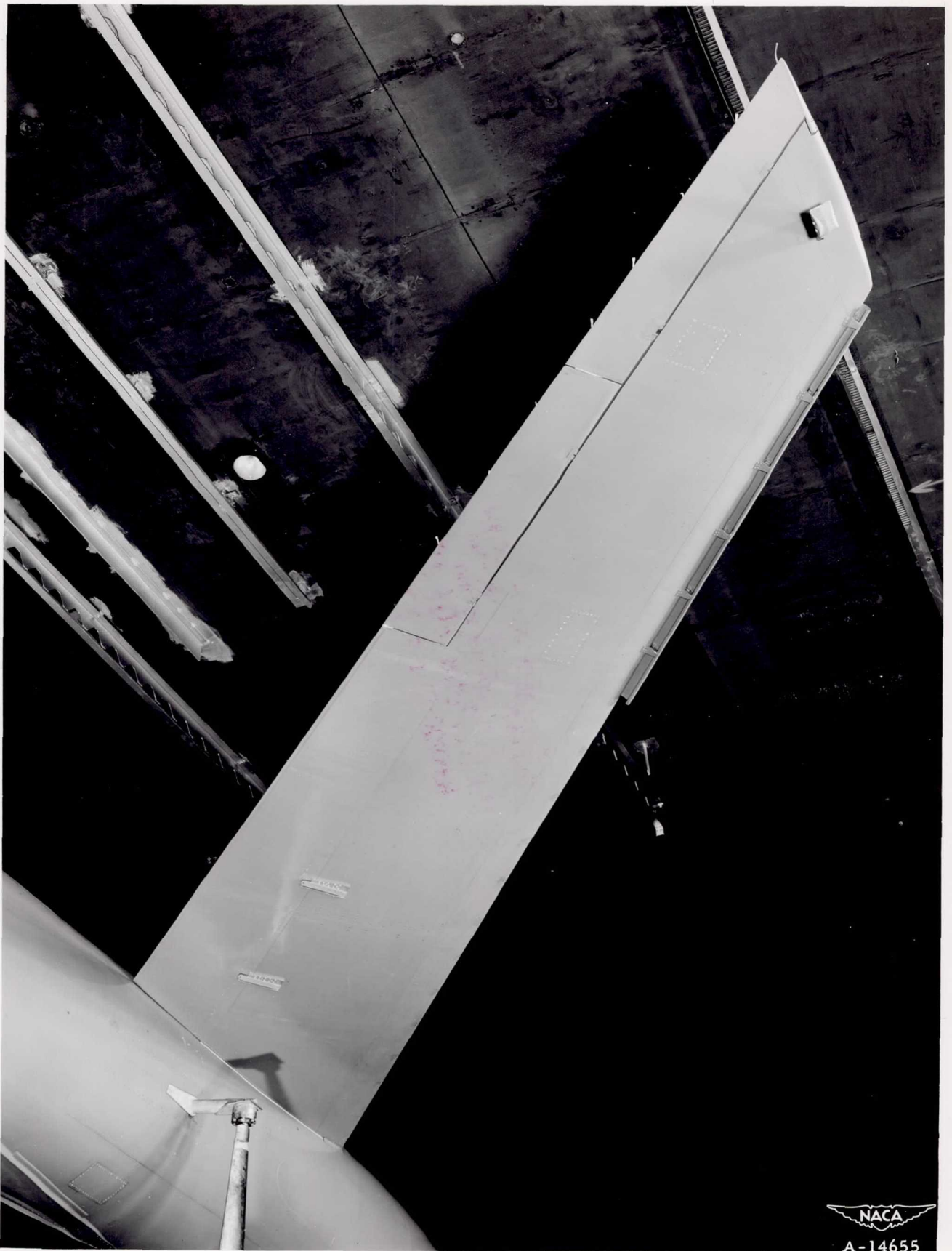
(e) Close-up of lower surface of right wing with 30-percent-span leading-edge flap.
