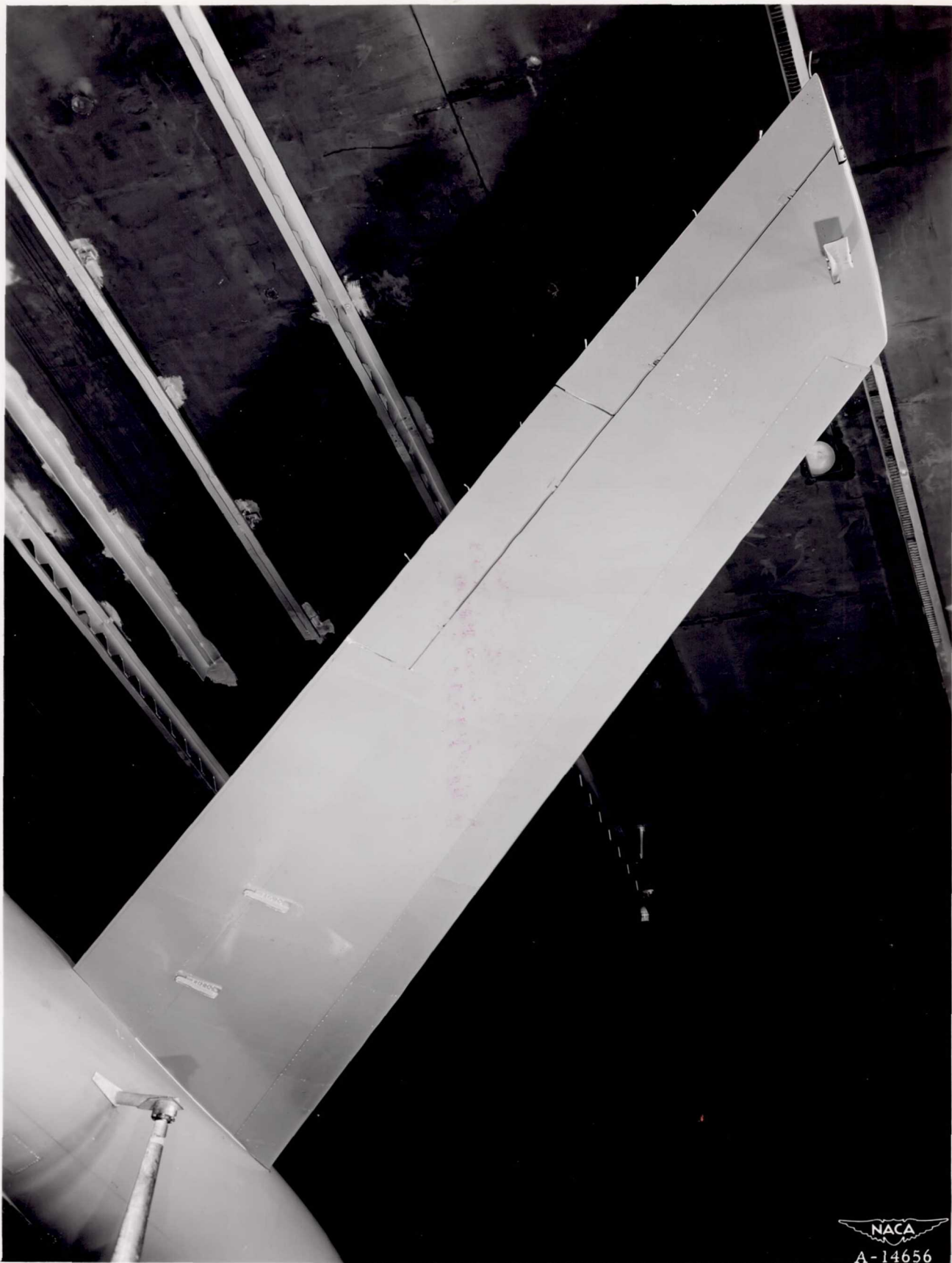
(f) Close-up of lower surface of right wing with increased leading-edge radius.
