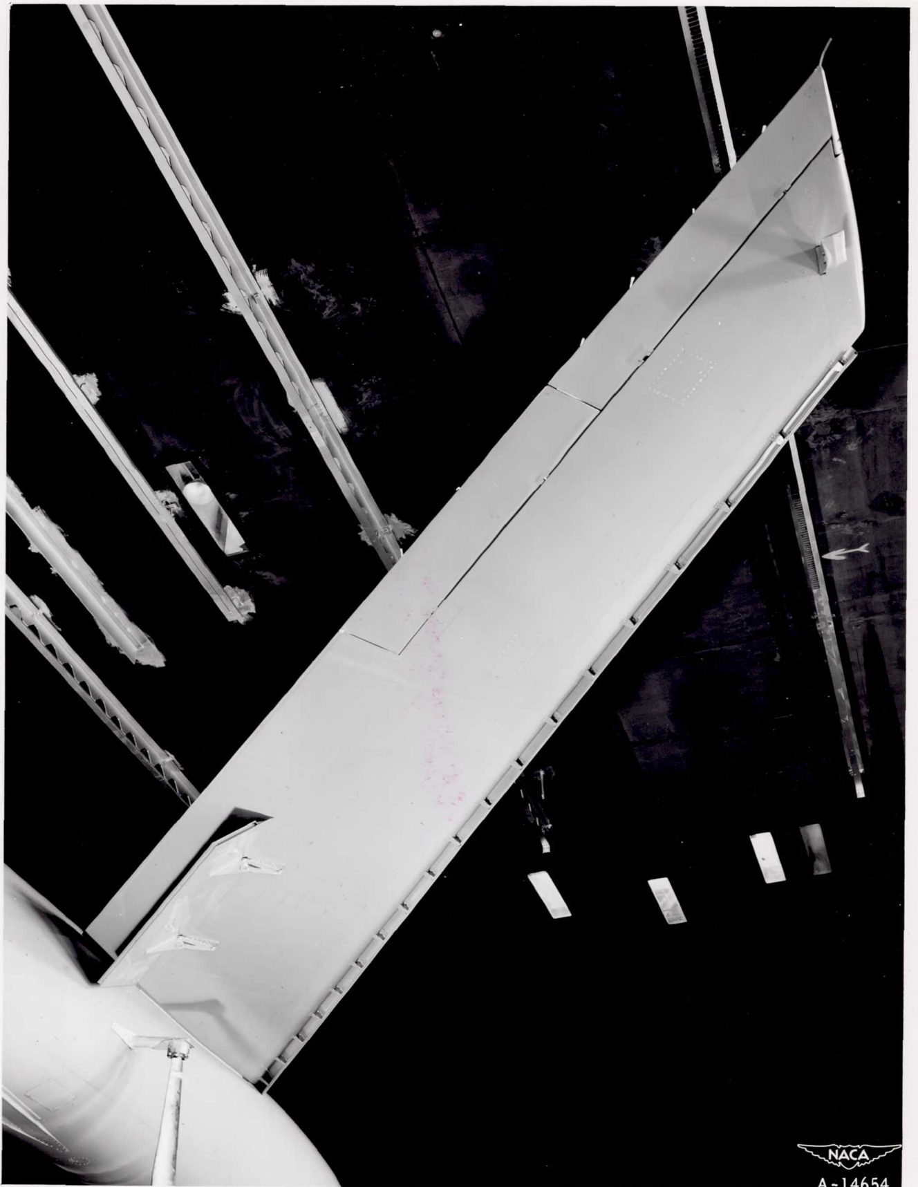
(d) Close-up of lower surface of right wing with full-span leading-edge flap and trailing-edge flap deflected 45^\circ .
