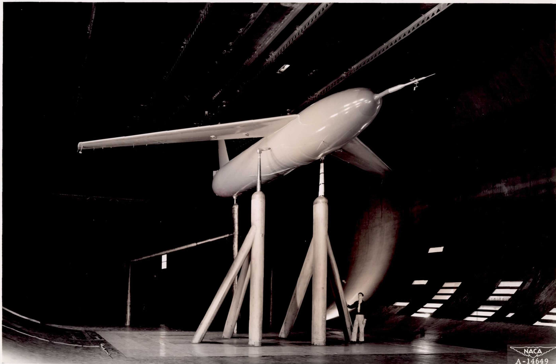
(g) General view of model with increased leading-edge radius.
