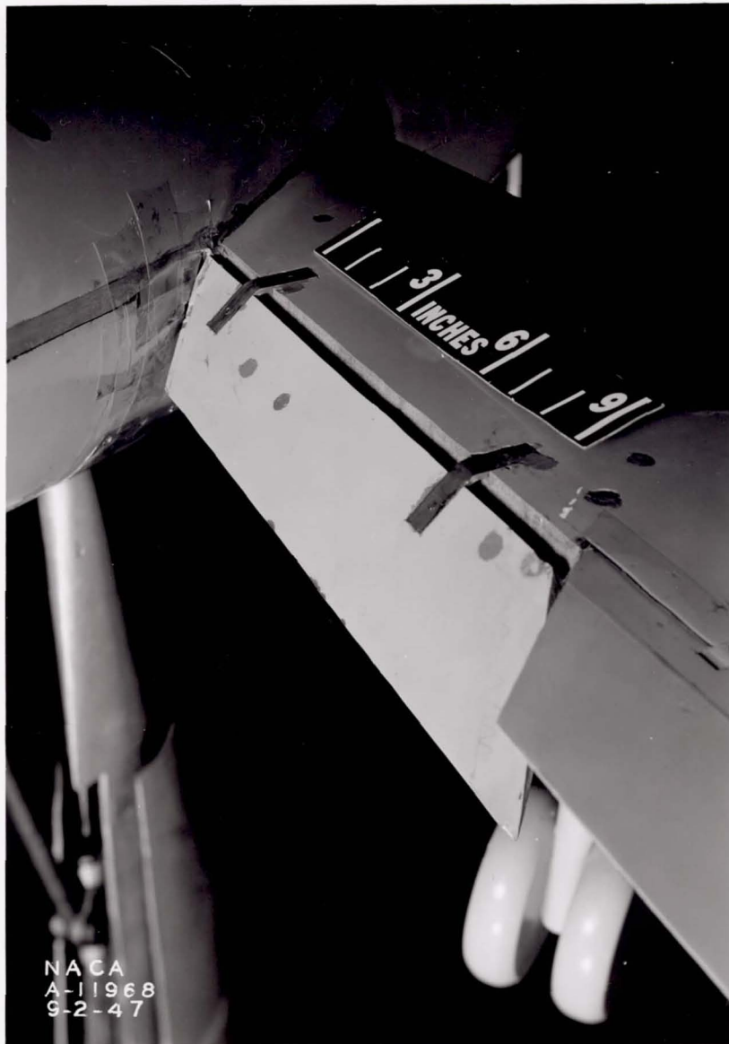
Figure 16.- Detail of plain flap.
