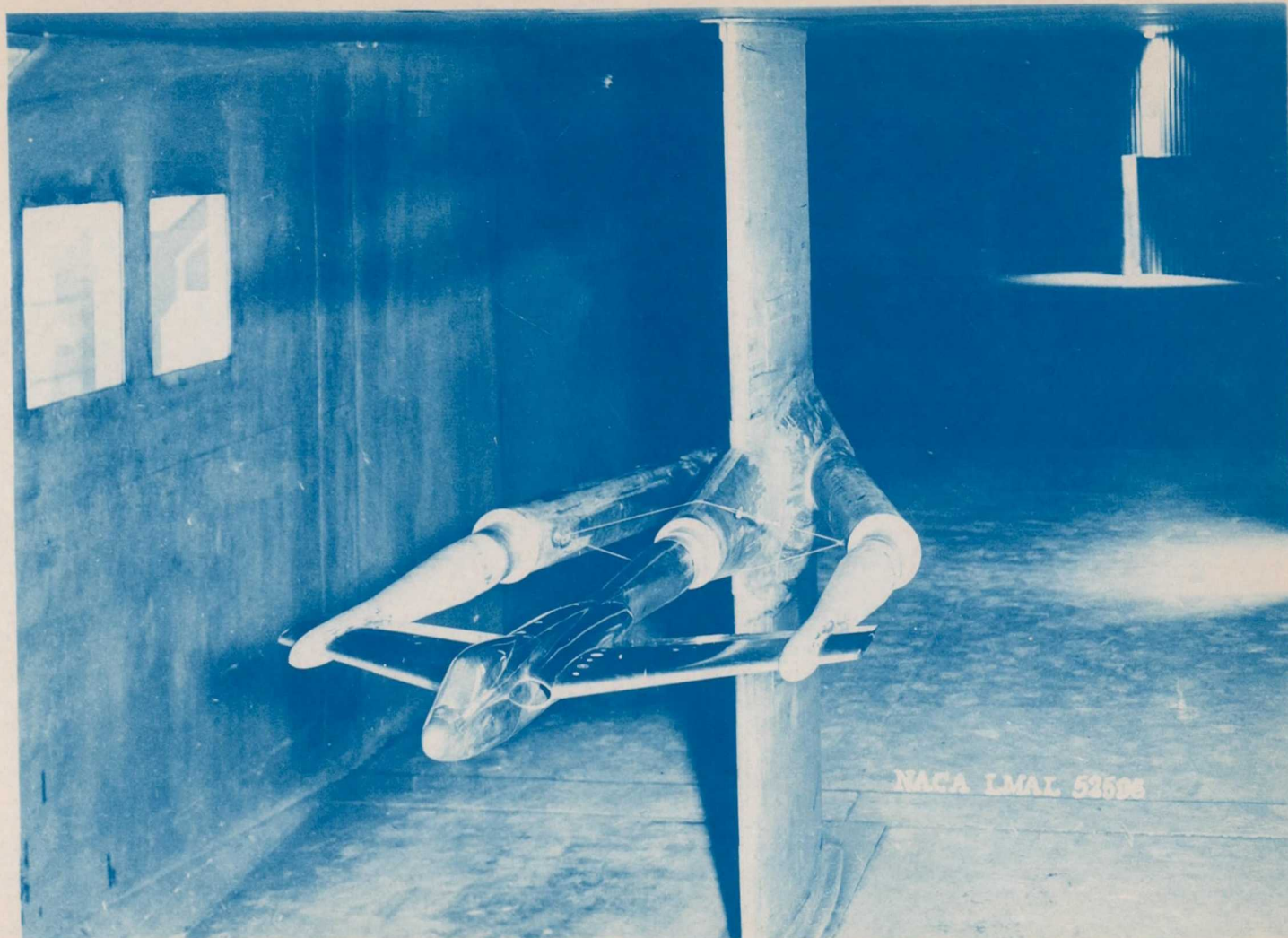
Figure 4.- Photograph of the 0.08-scale model of the XF7U-1 airplane with vertical tails removed mounted on the wing supports with center sting in place.
