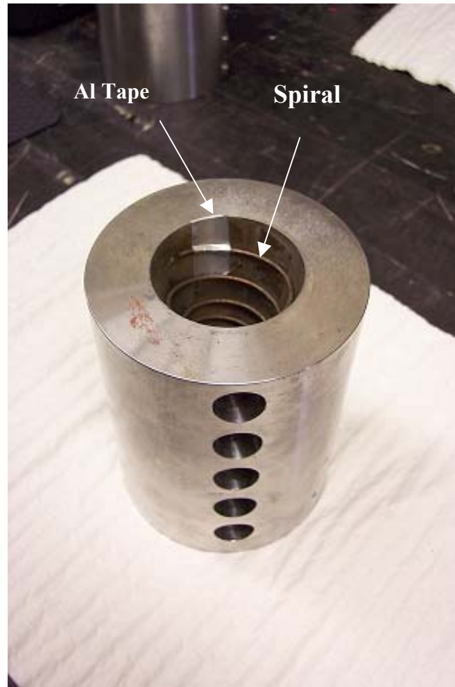
Figure 11. Shchelkin spiral installed in a detonation actuator.
