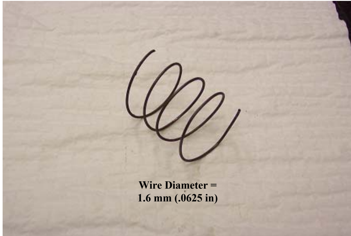
Figure 10(b). Shchelkin spirals used in the constant area tube.
