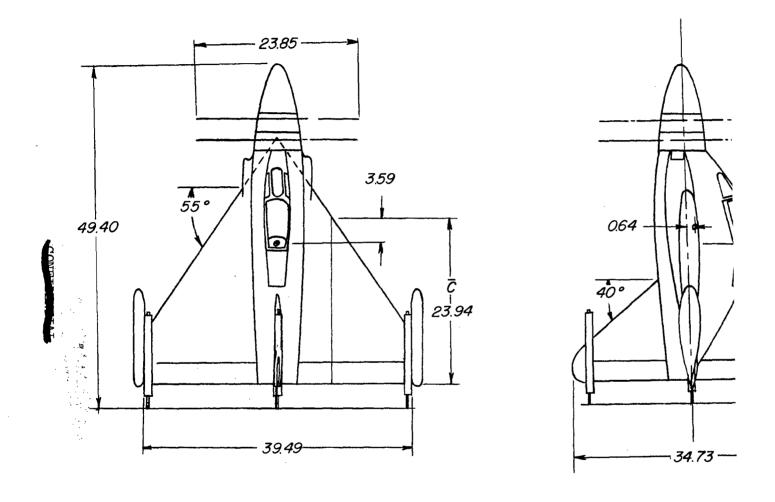
Figure 4.- The Convair XFY-1 vertically rising airplane model. Al dimensions are in inches.
