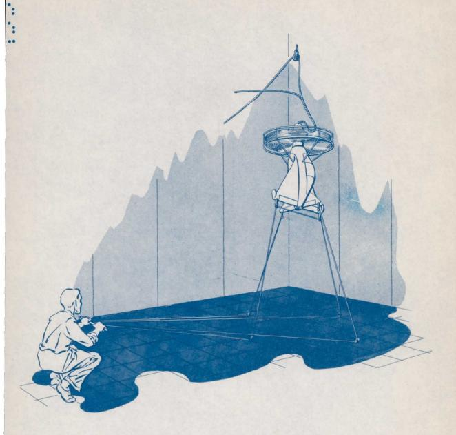
Figure 1.- Tethering system proposed by Convair.
