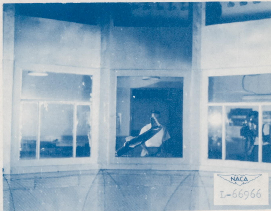
Figure 10.- Photograph of the \frac{1}{24} -scale model of the Grumman AF-2S airplane equipped with the original tail spinning in the Langley 20-foot free-spinning tunnel.
