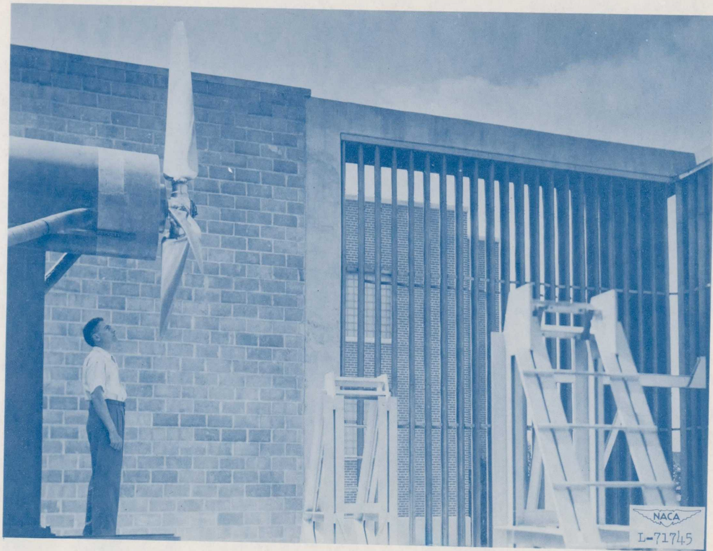
Figure 1.- The 6000-horsepower propeller dynamometer without model. Configuration II.
