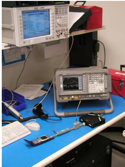
Figure A.4: QUALCOMM Radiated Emissions Test Setup in GPS Band Test Setup
