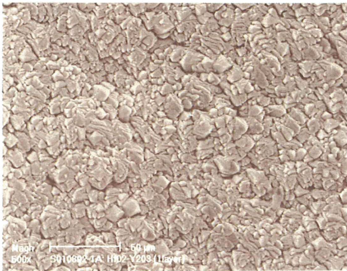
SEM micrographs showing the surface morphology of HfO 2 – 27 wt% Y 2 O 3 (PCR - 1 layer) deposited on platinum aluminide - coated MAR-M-247. Sample # S010802-1A
