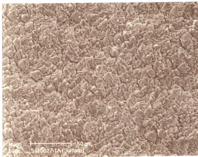
SEM micrographs showing the surface morphology of \text{HfO}_2 - 27\text{wt}\% \text{Y}_2\text{O}_3 (PCR 40 layer) deposited on platinum aluminate-coated MAR-M-247. Sample # S010627-1A
