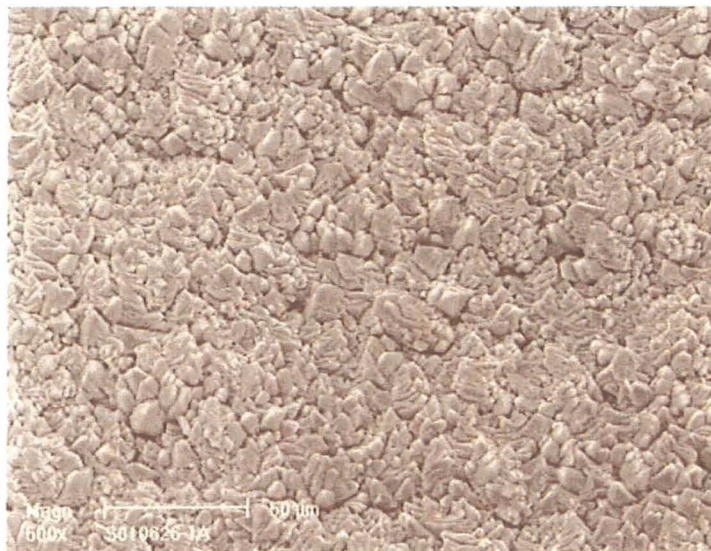
SEM micrographs showing the surface morphology of \text{HfO}_2 - 27\text{wt}\% \text{Y}_2\text{O}_3 (PCR-1 layer) deposited on platinum aluminide-coated MAR-M-247. Sample # S010626-1A
