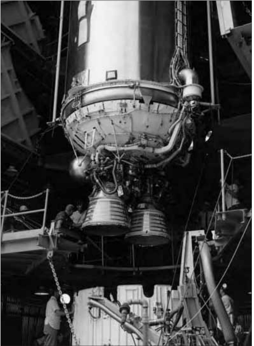
Technicians at Pad 36A gingerly lower Centaur into the interstage adapter on top of Atlas, August 1964. (KSC 64-16746)
