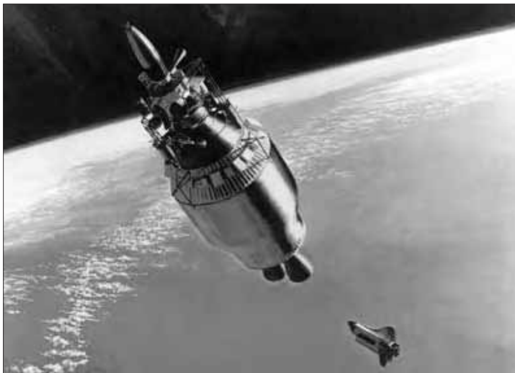
Artist's rendering of the Shuttle/Centaur. The Centaur and its payload have separated from the Shuttle and are preparing to launch after the Shuttle flies away to a safe distance. (Glenn Research Center unprocessed photo)
