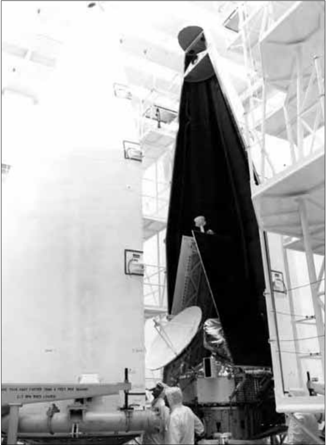
Mariner Venus/Mercury 10 is prepared for encapsulation on 21 September 1973 at Kennedy Space Center. (NASA KSC_73P_0541)
