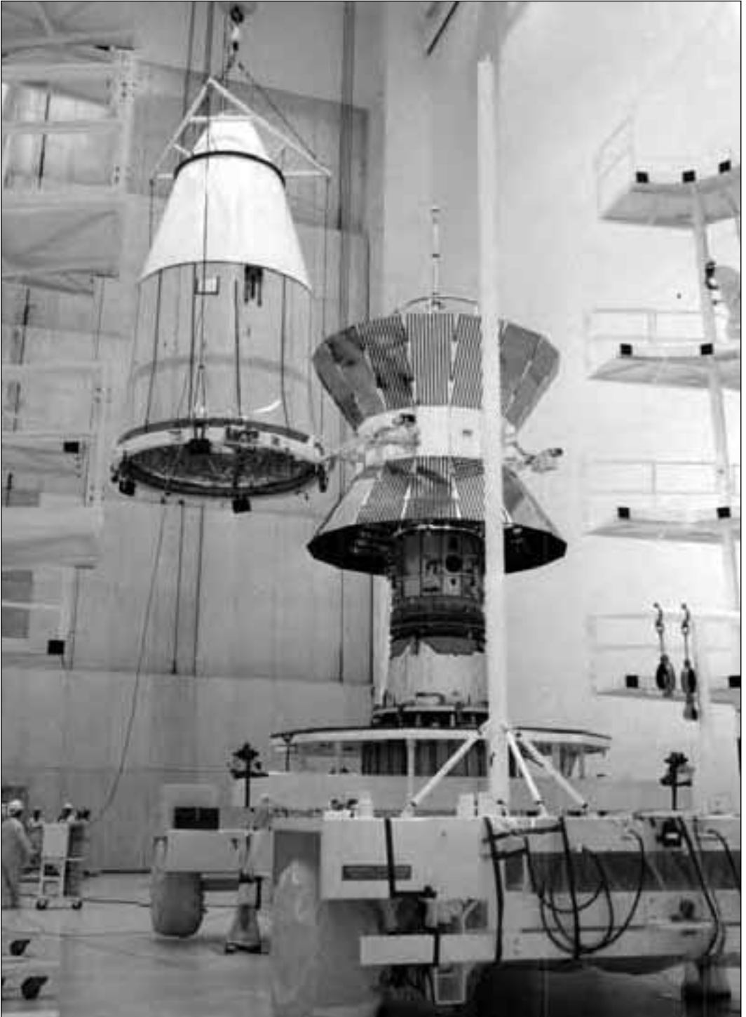
A Helios spacecraft prototype is encapsulated in its payload fairing at Kennedy Space Center on 27 September 1974. This work was in preparation for a future Titan-Centaur flight. (NASA KSC_74P_0222)
