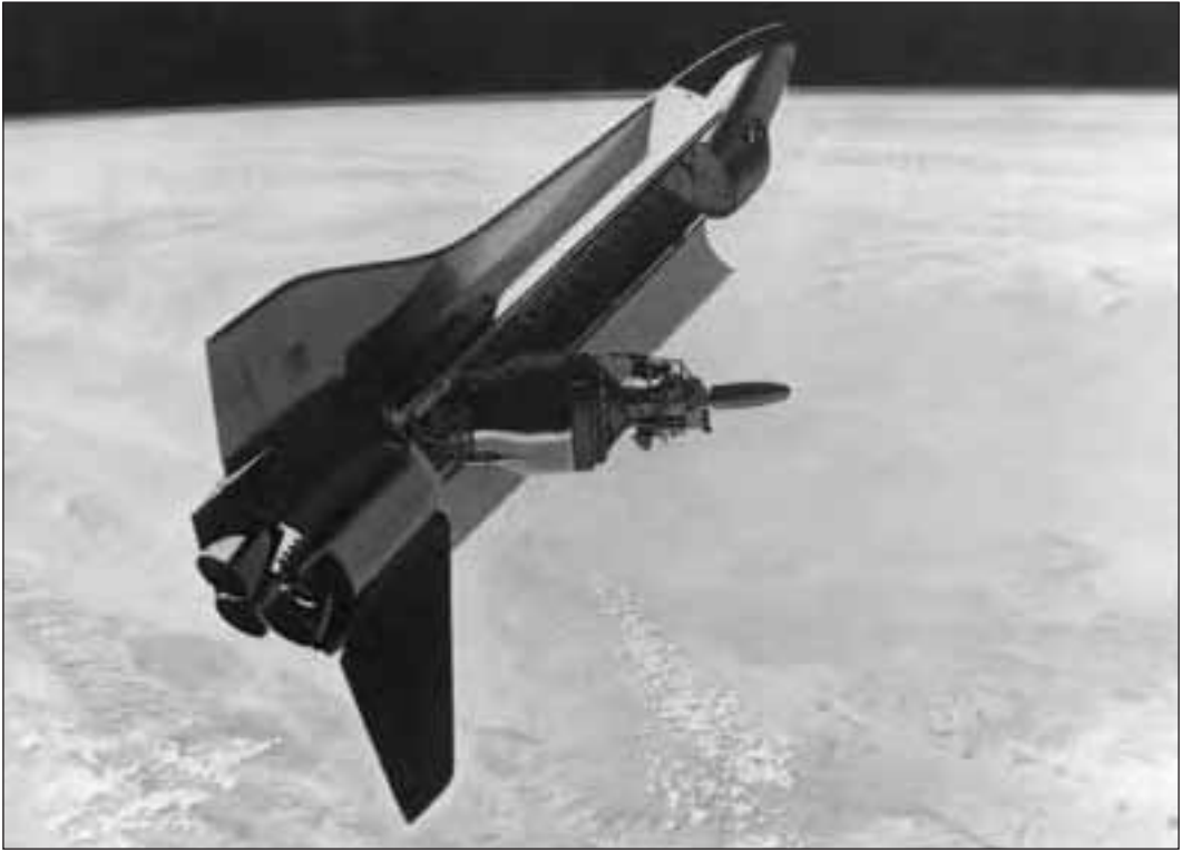
Artist's rendering of Shuttle/Centaur preparing to launch payload. The bay doors are open, and the payload is about to be released by the Centaur Integrated Support Structure (CISS). (Glenn Research Center unprocessed photo)
