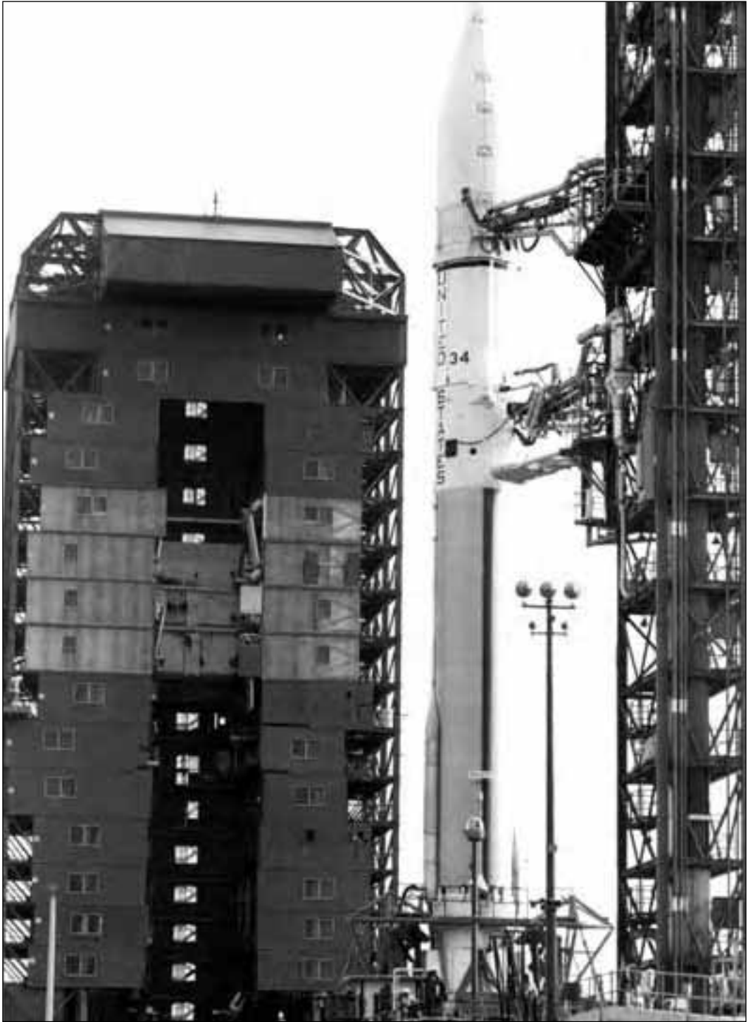
Atlas-Centaur 34 undergoing a tanking test on NASA Complex 36B at Cape Kennedy. This launch was the first dual-planet flight, Mariner Venus/Mercury 10. 19 September 1973. (NASA KSC_73P_0537)
