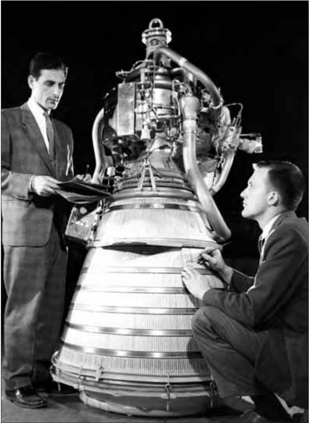
NASA engineers Ali Mansour and Ned Hannum review test results of Pratt & Whitney's RL10 engine at Lewis Research Center, 1963. (NASA C-64329)
