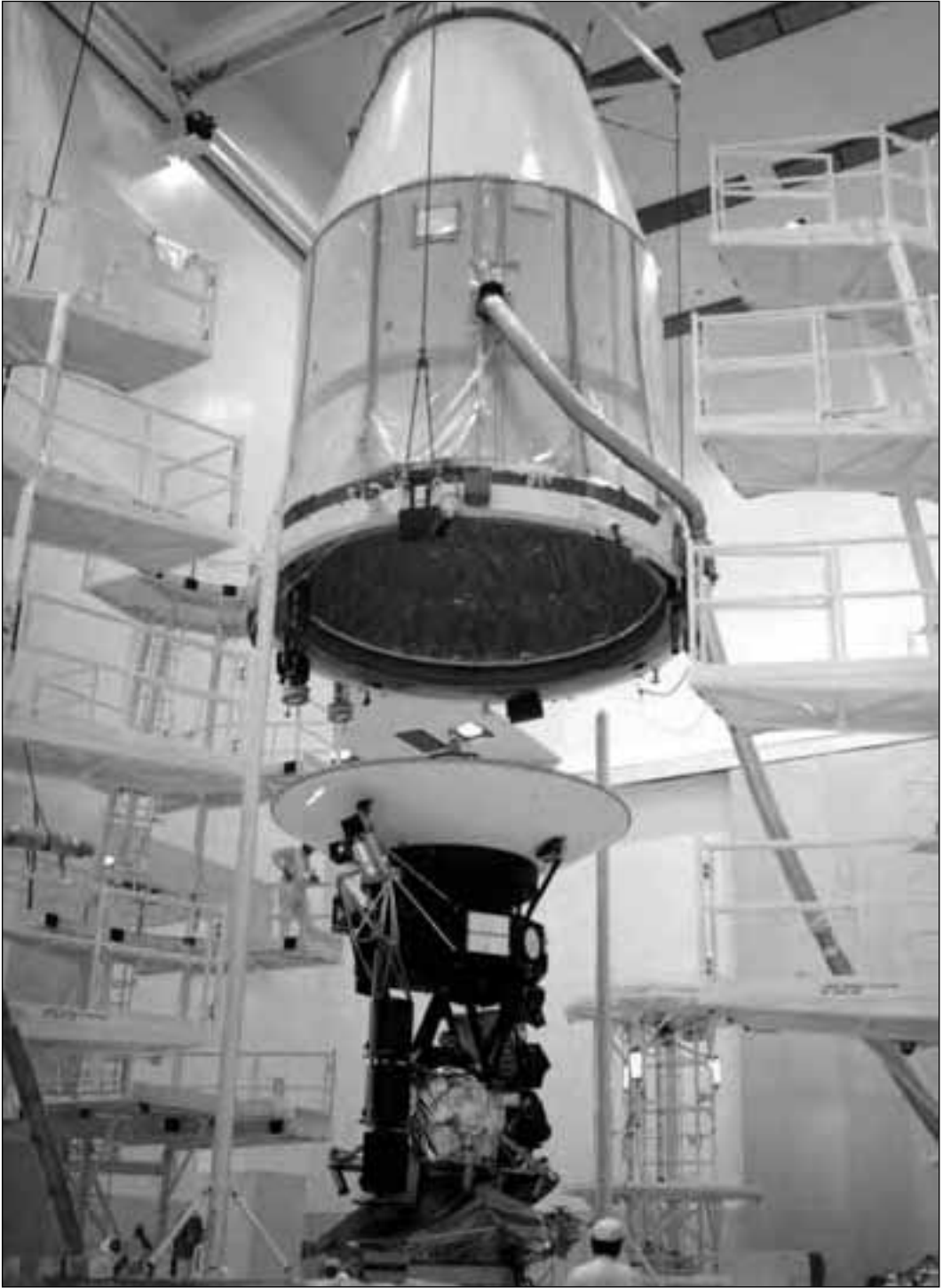
The Voyager spacecraft as it is encapsulated within its protective shroud at the Spacecraft Assembly and Encapsulation Facility at Kennedy Space Center on 2 August 1977. It would later be mated with Titan-Centaur 7 for launch on 20 August 1977. (NASA KSC_77P_0201)
