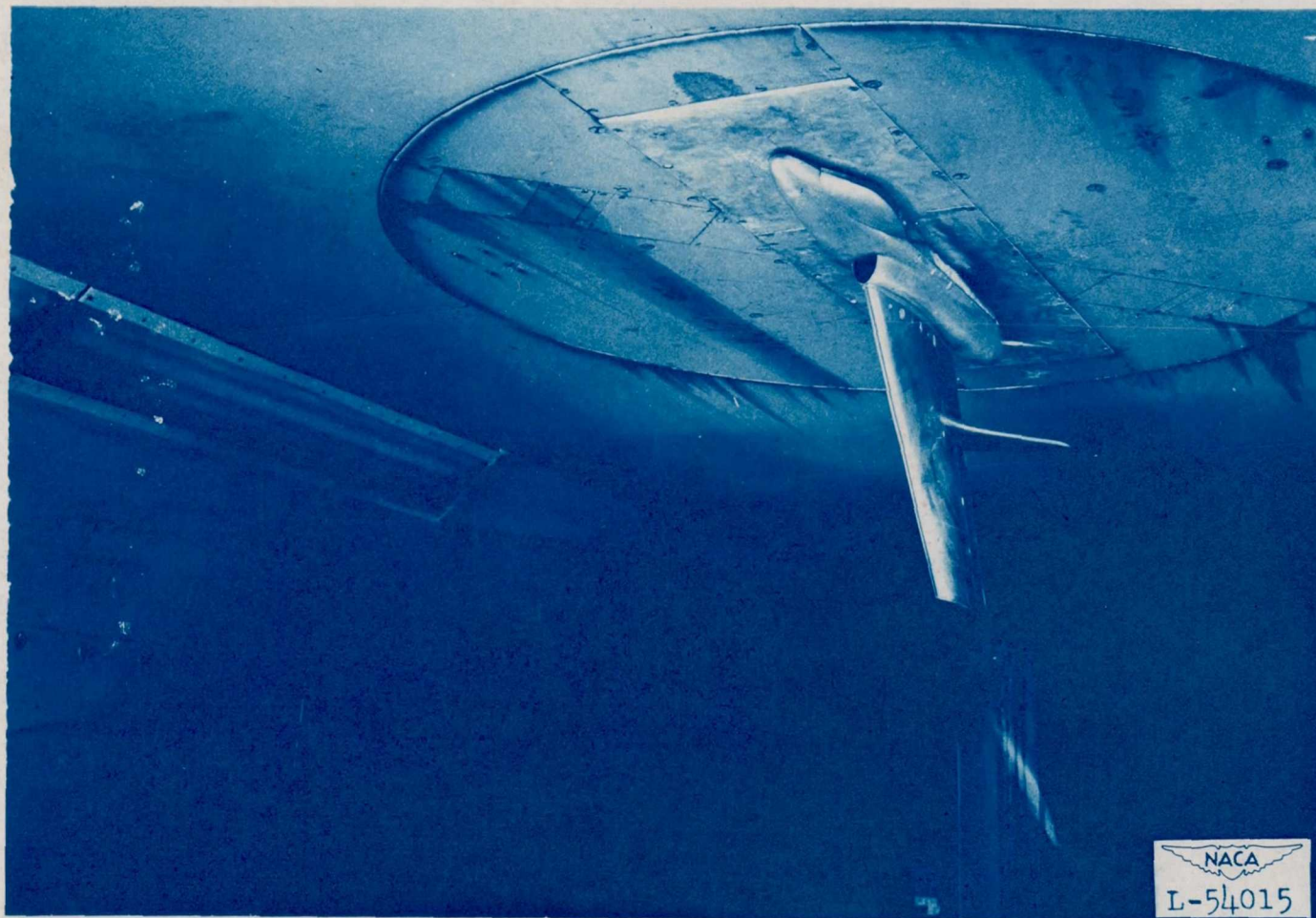
Figure 3.- The 0.08-scale semispan model of the XF7U-1 airplane with vertical fin on, mounted on the Langley 7- by 10-foot high-speed tunnel ceiling.
