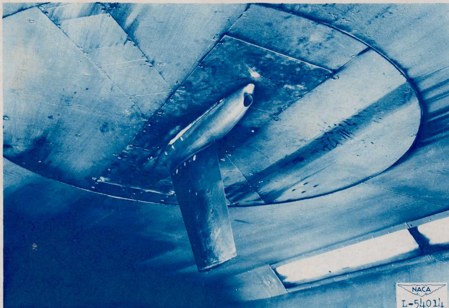
Figure 4.- The 0.08-scale semispan model of the XF7U-1 airplane with vertical fin removed, mounted on the Langley 7- by 10-foot high-speed tunnel ceiling.
