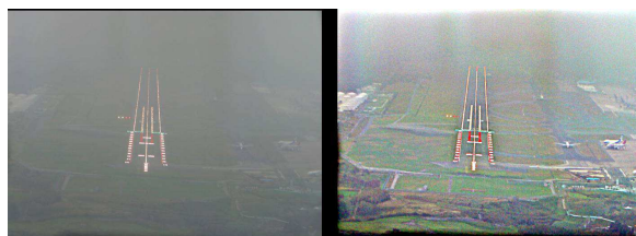
Figure 1. Original image of a runway on the left; Retinex enhanced image on the right. Note the improvement in visibility of the runway and surrounding areas.
