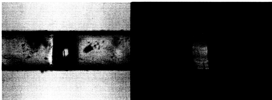
Tetragonal lysozyme covalently labeled (0.5% of the protein) with the fluorescent probe PyMPO (Molecular Probes, catalog S-611) in a 0.3 mm capillary under white light (left) and fluorescent (right) illumination.
