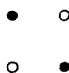
Fig. 7. Square lattices can be formed by using particles of two "spins". Unlike spins are R apart while like spins are \sqrt{2}R apart.
