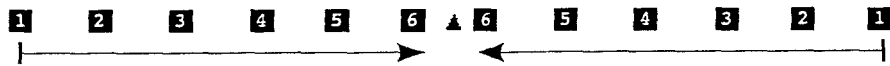
Fig. 4. Simulation of a fluxotaxis-driven lattice (represented by black boxes) in the vicinity of a chemical source from the Divergence Lemma 1. The time trace, denoted by the numbered boxes, shows the location of each of the two different agent lattices at sequential time steps in the simulation. Both lattices correctly converge on the true location of the chemical emitter
