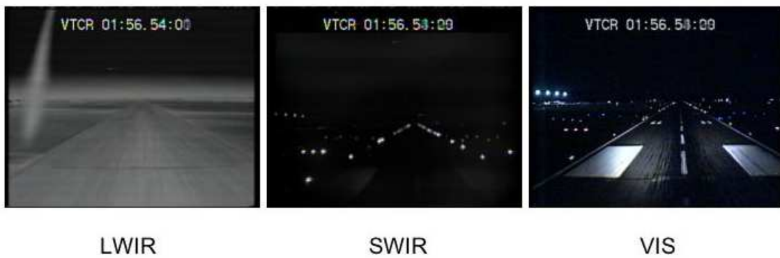
Figure 3. Examples of the imagery generated by each camera in good weather conditions. The images from cameras must be registered, enhanced, fused and displayed to the pilot in real-time.
