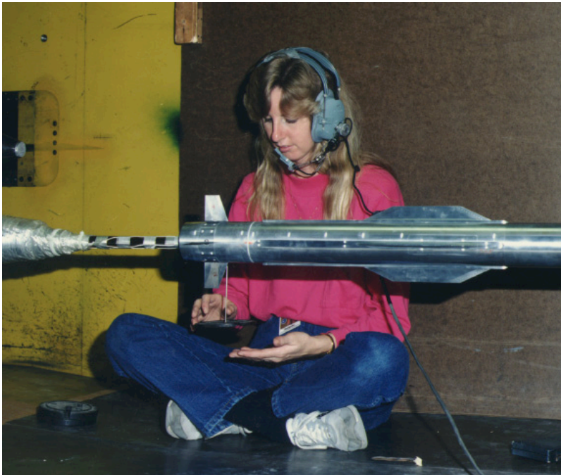
Figure 17. Tail fin check loads being applied to configuration 7 in test section 2 of UPWT.
