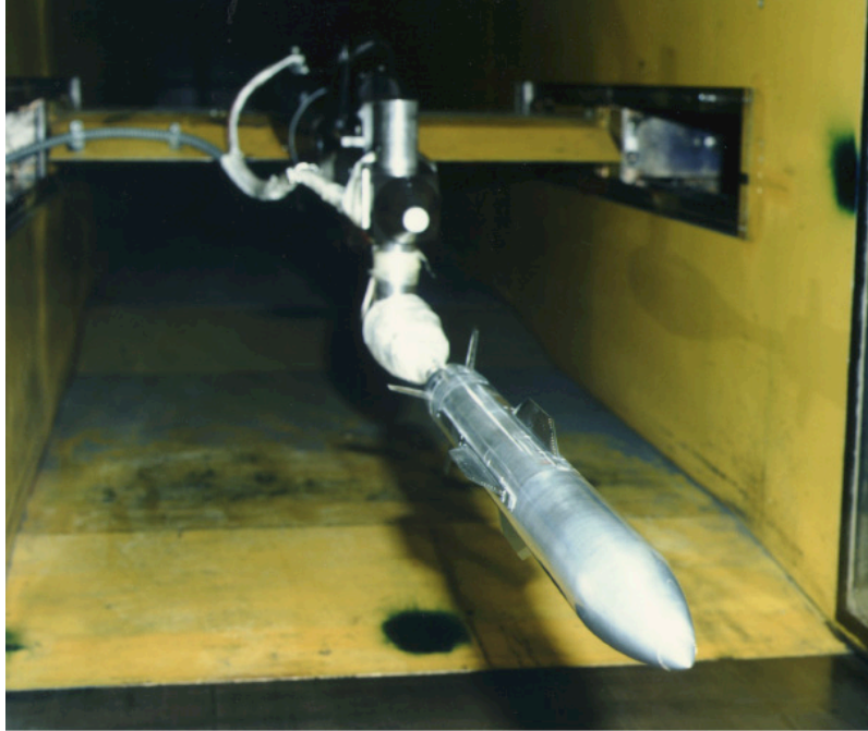
Figure 16. Configuration 7 in UPWT test section 2 showing model mounting setup.
