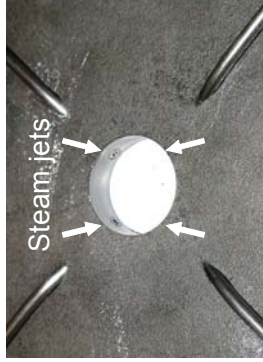
Specimen holder and water vapor jets
