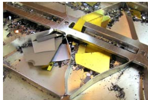
Fig. 2. Collector fragments trapped in array frame. Field of view is 15 cm.
