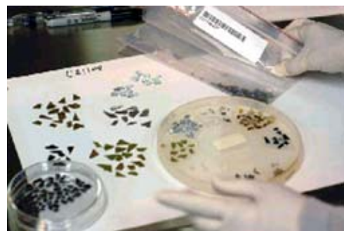
Fig. 3. Sorting shards by material type.
