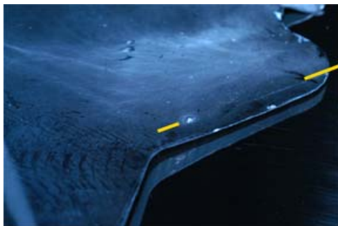
Fig. 5. Oblique lighting reveals dust or coatings on surface. Bright spot near center is mud/salt spatter. Between yellow lines a boundary mark exists corresponding to shadowing or impact imprint of saddle thermal shield.
