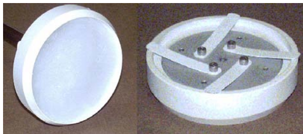
Fig. 1. a) (Left) Laboratory prototype version of the TGIP loaded with silicone grease. b) (Right) Backside of the TGIP collector. Springs and retractable outer ring are visible.
