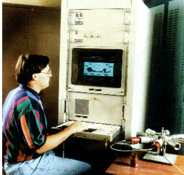
Leak-monitoring system with visual display of leak location.
