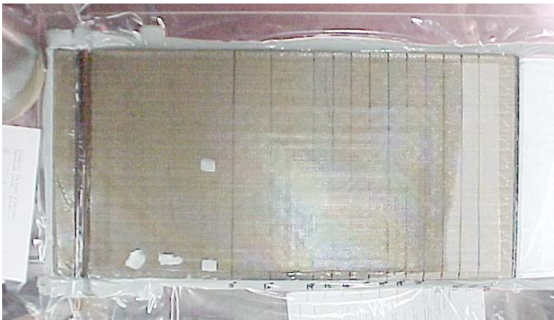
Figure 6.24: Top surface of stitched foam core preform with 12.7 mm stitch row spacing. Flow front is approximately 55.9 cm from injection edge
