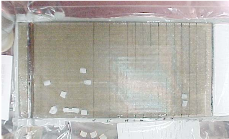
Figure 6.25: Top surface of stitched foam core preform with 12.7 mm stitch row spacing. Flow front is approximately 61.0 cm from injection edge
