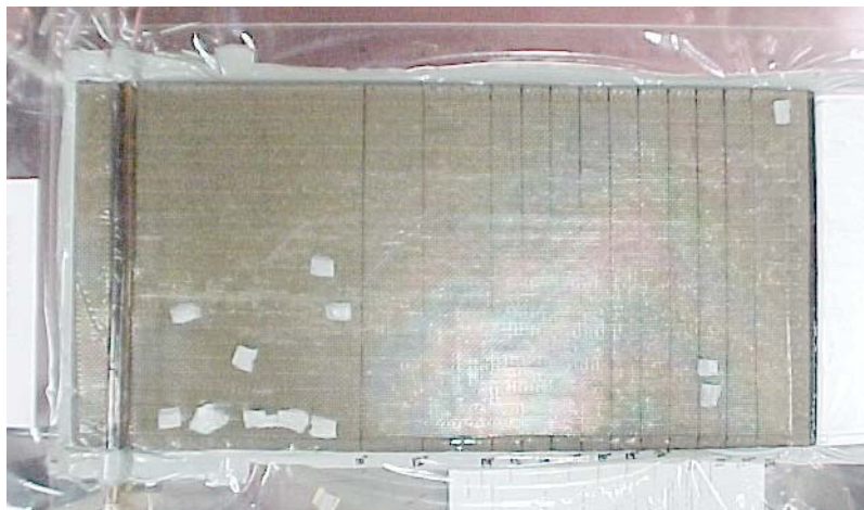
Figure 6.26: Top surface of stitched foam core preform with 12.7 mm stitch row spacing. The preform has been completely infiltrated
