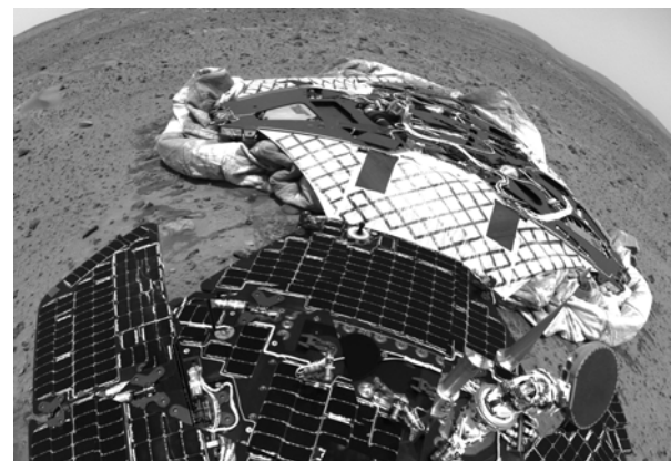
Figure 3: Navcam mosaic acquired immediately after the Spirit rover egress from the lander.
