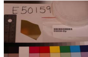
Figure 6: Wafer fragment with scale and color bars as well as the inventory tracking number and container.
