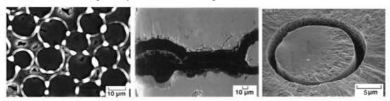
Oxidation behavior of model composites with BN layers. Top: At 816 °C for 100 hr with low water vapor, BN deposited at a low temperature forms borosilicate. Middle: At 900 °C for 140 hr with low water vapor, BN deposited at a high temperature remains intact. Bottom: At 500 °C for 100 hr with water vapor, BN deposited at a low temperature is volatilized.
