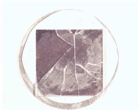
Figure 19.—Molybdenum and sapphire after hot press run at 1700 °C for 2 hr.
