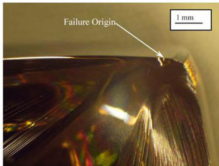
Figure 14.—View of fracture surface (J. Salem, NASA Glenn) on sapphire crystal tested on March 31, 2004. Note fracture origin near surface (ref. 2).
