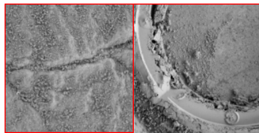
Fig.2 Microscopic images: left, as-is-surface at Sabre; right, abraded hole at Mastodon (frame size ~ 3 cm).
