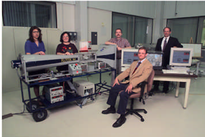
Small wind tunnel (6- by 6-in. test section) controlled over the Internet.
