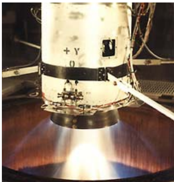
Rocket Engine Firing Inside Vacuum Test Cell
