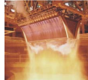
240 Klb Aerospike ... 17 tests (1999-2001)
