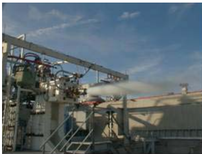
Subscale Ox-Rich Preb ... 15 tests (RS-76: Nov 98 – Jan 99) (RS-84: Fall 2003)
