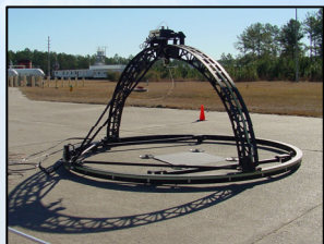
Sandmeier Field Goniometer for Bidirectional Reflectance Measurement
