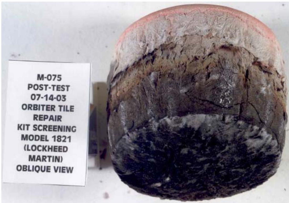
JSC2003E47270 – Model #1821, Post-Test, Front Oblique View
