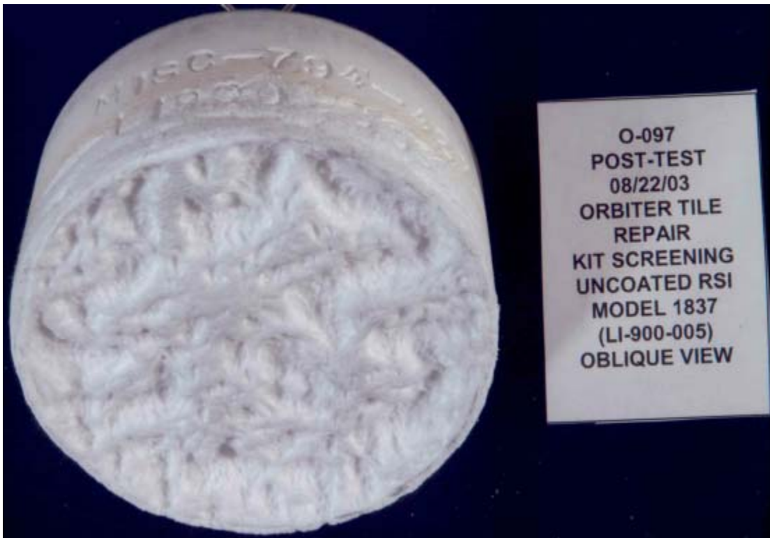
JSC2003E55041 – Model #1837, Post-Test, Front Oblique View
