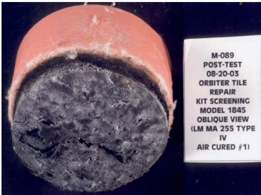
JSC2003E54541 – Model #1845, Post-Test, Front Oblique View
