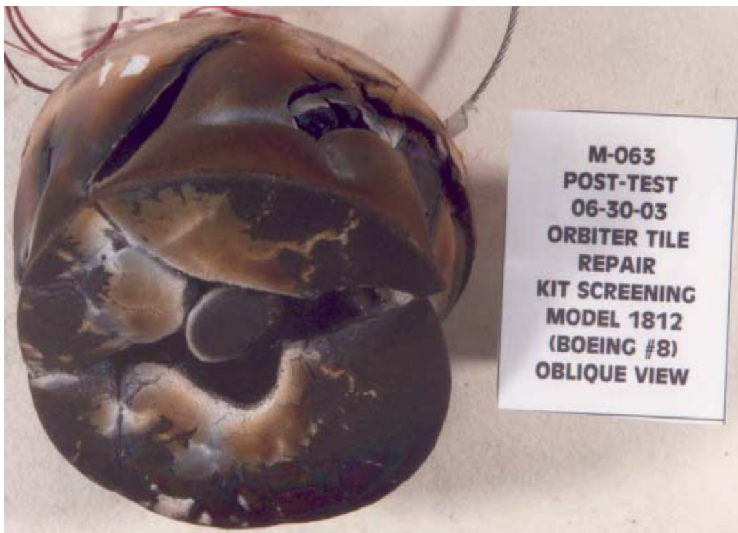
JSC2003E46687 – Model #1812, Post-Test, Front Oblique View
