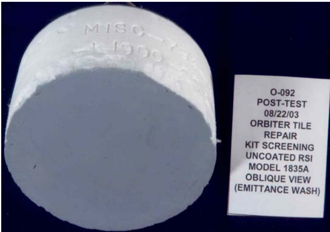
JSC2003E55046 – Model #1835A, Post-Test, Front Oblique View
