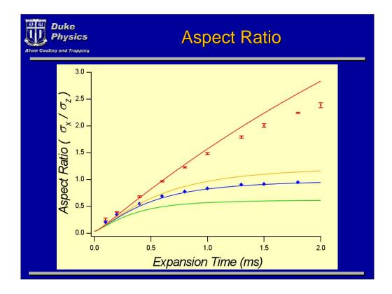
This is a plot of the measured aspect ratio as a function of time (red dots with error bars). The red line which closely approximates the data is for purely hydrodynamic expansion with no free parameters.
