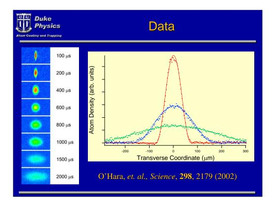
This plot shows the expansion of the initially narrow dimension as a function of time. It is quite clear that this direction expands much more rapidly than the long dimension.
