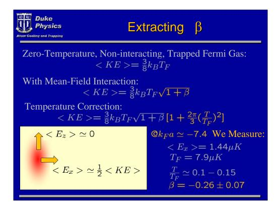
We can extract a measurement for  $\beta$  from our data by relating the kinetic energy of the released cloud to its size after expansion. We account for the finite temperature of the cloud with a Sommerfeld expansion of the density and for the mean-field interaction using the parameter  $\beta$ .
