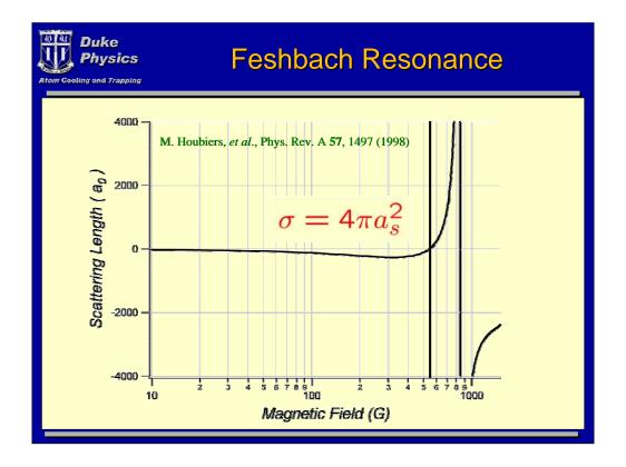
This plot shows the s-wave scattering length as a function of magnetic field for the two lowest hyperfine groundstates of <sup>6</sup>Li. Two Feshbach resonances are shown, a narrow resonance at approximately 550G and a very broad resonance centered near 850 G.
