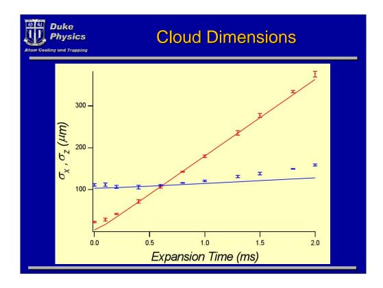
The previous slide showed that hydrodynamic expansion seemed to explain the observed data, however there was a non-negligible deviation at long times. This plot shows the growth of both the initially narrow (red) and initially long dimensions of the cloud.
