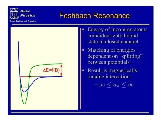
Strong interatomic interactions are produced in the system by a Feshbach resonance. In a Feshbach resonance, the energy of the colliding atoms is energetically tuned into resonance with a bound state on a closed exit channel. In <sup>6</sup>Li, the two relevant channels are the single and triplet potentials. The triplet state tunes in a magnetic field, so the relative spacing between the potentials can be varied by changing an externally-applied magnetic field.
