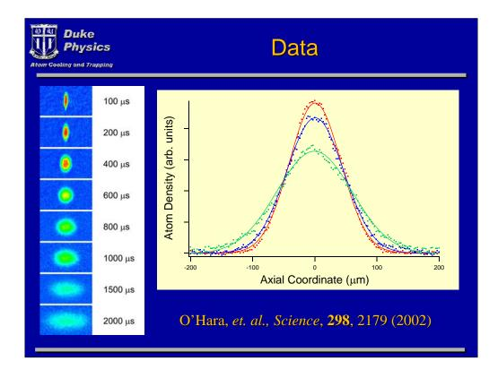
We can release the cloud for varying times and then image using absorption imaging to get the profile of the atomic cloud. The cloud starts in a long, cigar shape and expands in a very anisotropic manner. The narrow direction of the cloud expands quickly, while the initial long direction hardly moves.
