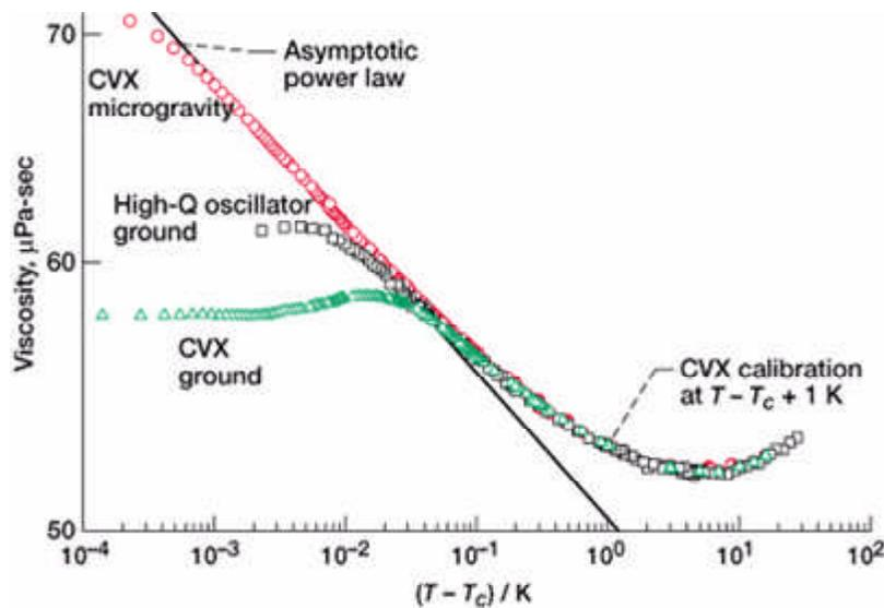
*Ground-based and microgravity measurements of the viscosity of xenon near the critical point. In microgravity, the increase of viscosity is measured 100 times closer to the critical temperature  $T_c$  and much more accurately than on Earth. The asymptotic power law characterizes the universal behavior of viscosity in all pure fluids near the critical point. Temperature of sample,  $T$ ; quality factor,  $Q$ . (High- $Q$  indicates weak damping.)*
