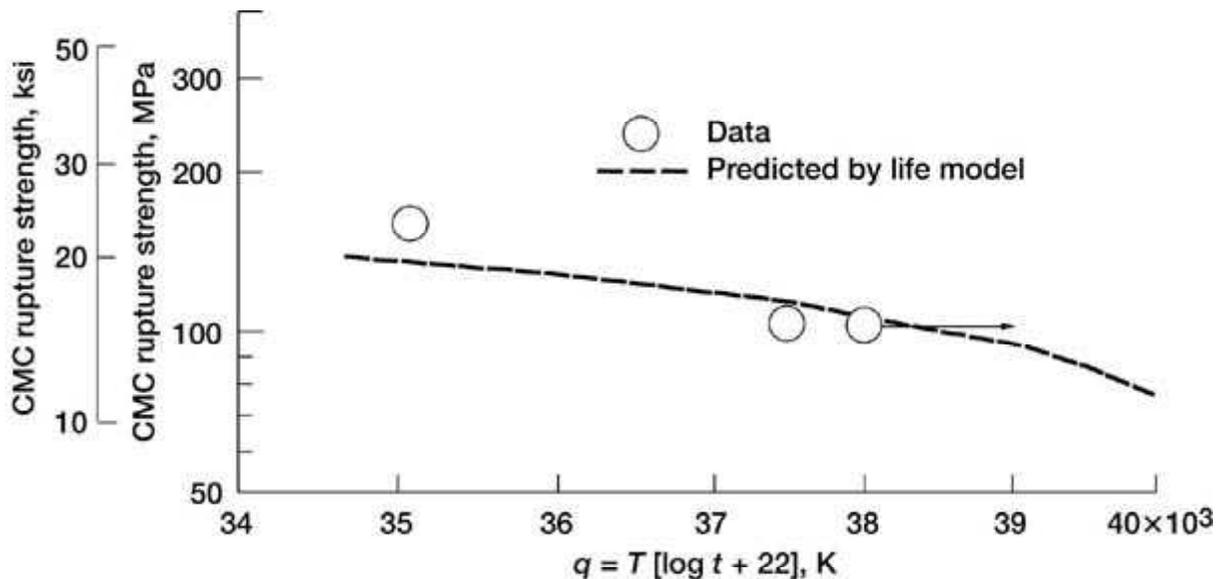
*Time- and temperature-dependent rupture strength for a state-of-the-art SiC/SiC composite.*
