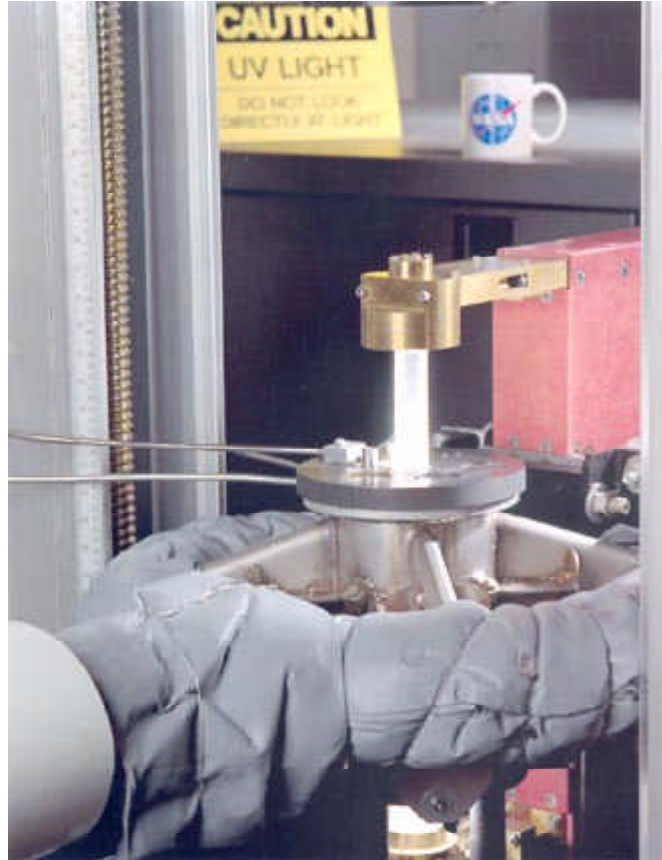
Electric plasma arc-lamp combustor liner durability test system.
