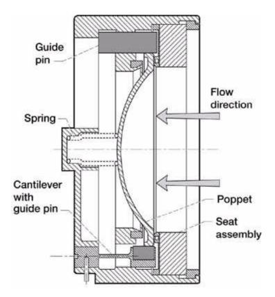
Potential application of CVD diamonds for valves such as the guide pins and seat assemblies in the space shuttles' check valves.
