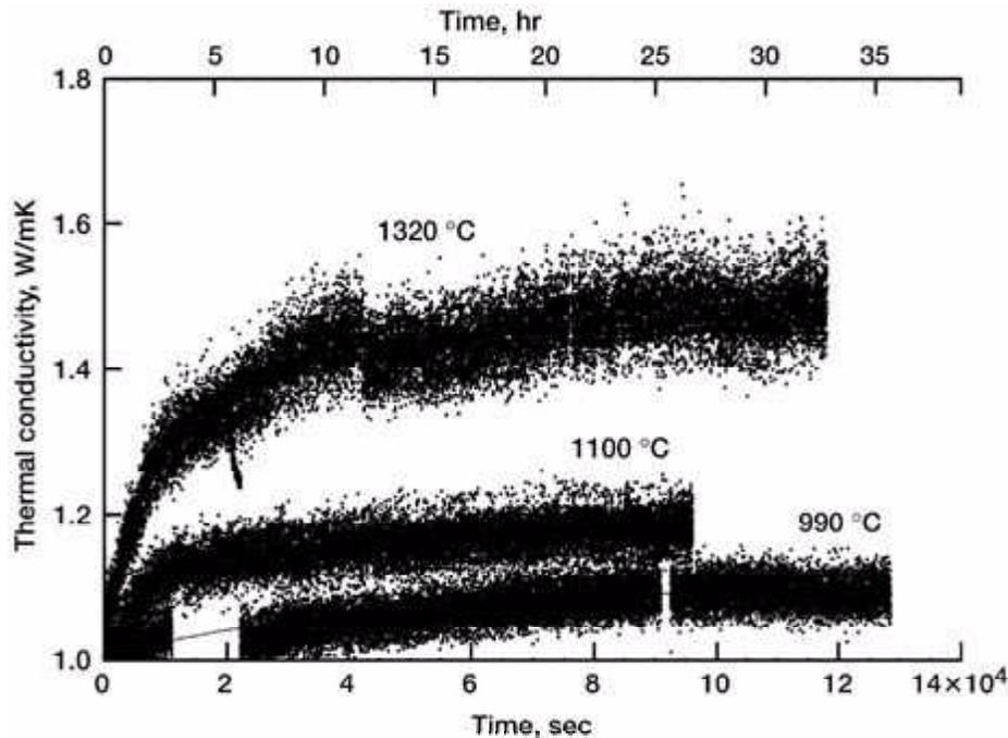
*Overall thermal conductivity change kinetics of the ZrO<sub>2</sub>-Y<sub>2</sub>O<sub>3</sub> thermal barrier coating determined by real-time laser heat flux testing.*
