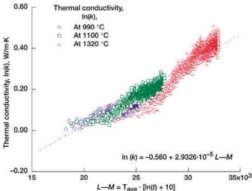
*Ceramic thermal conductivity  $\ln(k)$  as a function of Larson-Miller ( $L-M$ ) parameter ( $L-M = T_{ave}[\ln(t) + C]$ , where  $t$  is the heating time in seconds,  $T_{ave}$  is the average temperature in the ceramic coating in kelvin, and  $C$  is a fitting constant that equals 10 in this study). The effects of heating time and temperature on the overall ceramic thermal conductivity are approximately described by the conductivity to Larson-Miller relationship.*
