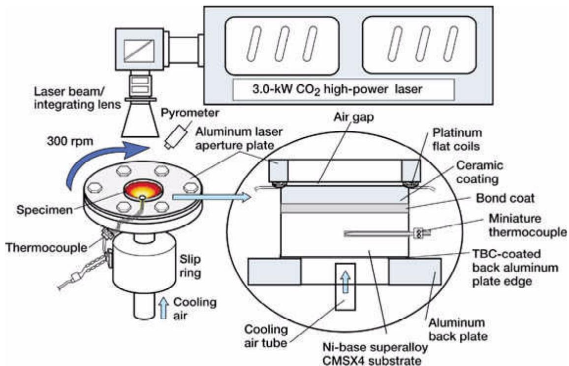
*Laser high heat flux rig for determining the thermal conductivity change kinetics of thermal barrier coatings. During the test, the ceramic surface and the metal backside temperatures are measured by infrared pyrometers. The metal substrate midpoint temperature can be obtained by an embedded miniature type-K thermocouple. The interfacial temperatures and the actual heat flux passing through the thermal barrier*
