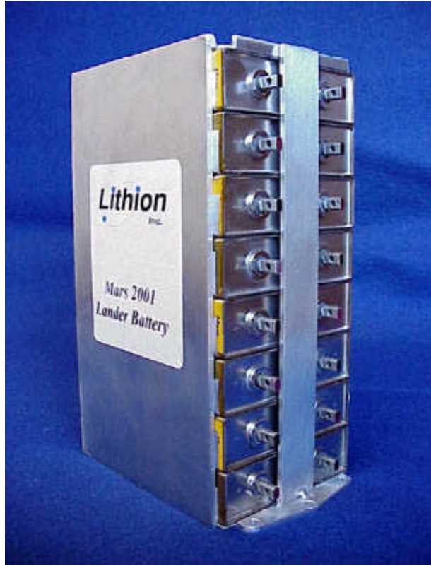
Prototype 25 A-hr, 28-V lithium-ion battery selected for Mars 2001 Lander.
