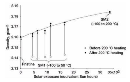
Density of pristine FEP and FEP retrieved from the Hubble Space Telescope during the first and second servicing missions, prior to and after heating at 200 °C for 7 to 9 days.
