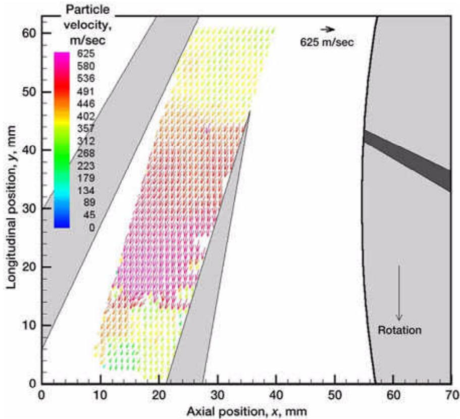
*The instantaneous velocity field captured during compressor surge. The velocity vector magnitudes are coded by color. The position of the impeller is shown on the right, and the diffuser vanes are shown on the left. Velocity measurements are obtained in the region of the flow field illuminated by the laser light sheet.*
