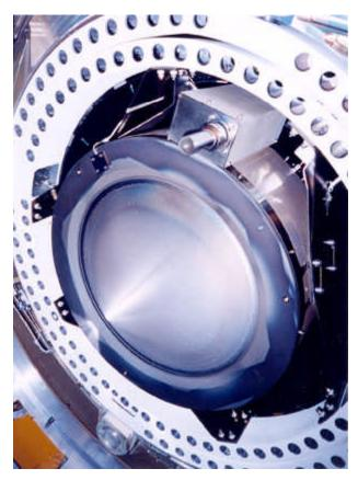
Flight ion thruster mounted to the Deep Space 1 spacecraft gimbal assembly.
