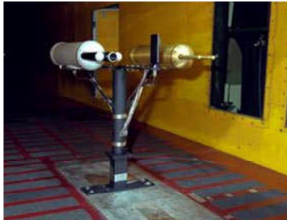
Particle sizing probes in Glenn's Icing Research Tunnel during NASA/Atmospheric Environment Service international SLD instrumentation comparison test.
