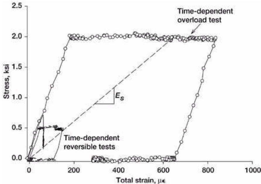
*Time-dependent deformation tests provide explicit determination of the reversible-irreversible threshold stress ( $\kappa = S_{\text{applied}} - \epsilon_{\text{IR}} E_s$ ) by using viscoelastic subtraction for a titanium alloy at 650 °C.*
