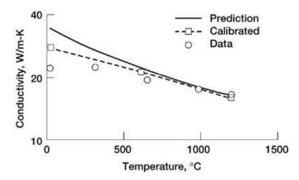
Through-the-thickness thermal conductivity. Constituents: F-34.1
