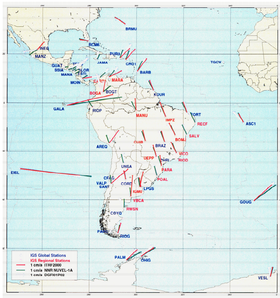
Figure 1: IGS RNAAC SIR network and horizontal velocities of solution DGFI01P02 compared with ITRF2000 and NNR NUVEL-1A
