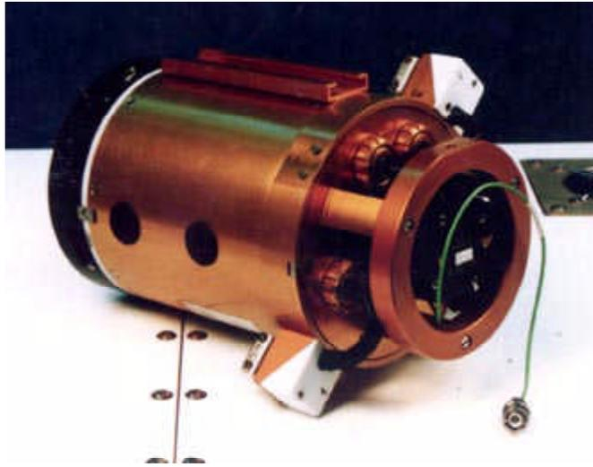
*ALICE II thermostat for critical fluid samples. It enables stable temperature control ( $\pm 50$  m°C rms) and optical diagnostics like interferometry and microscopy.*
