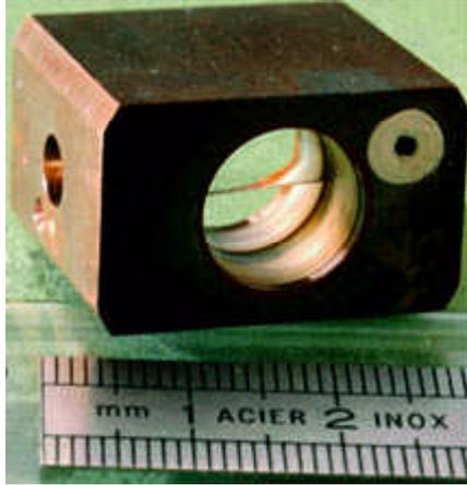
*Typical copper-bodied cell with sapphire windows. It is filled with SF<sub>6</sub> to roughly 38 atm and a density of 0.73 g/cm<sup>3</sup>. The typical fluid volume was less than 1 cm<sup>3</sup>.*
